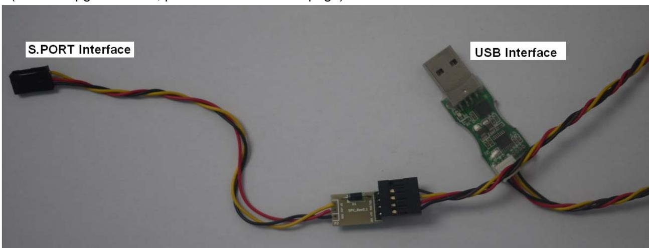
**Note: GND pin on SPC goes to BLACK wire of FrUSB-3/FUC-3 to make sure the connection is correct.**
