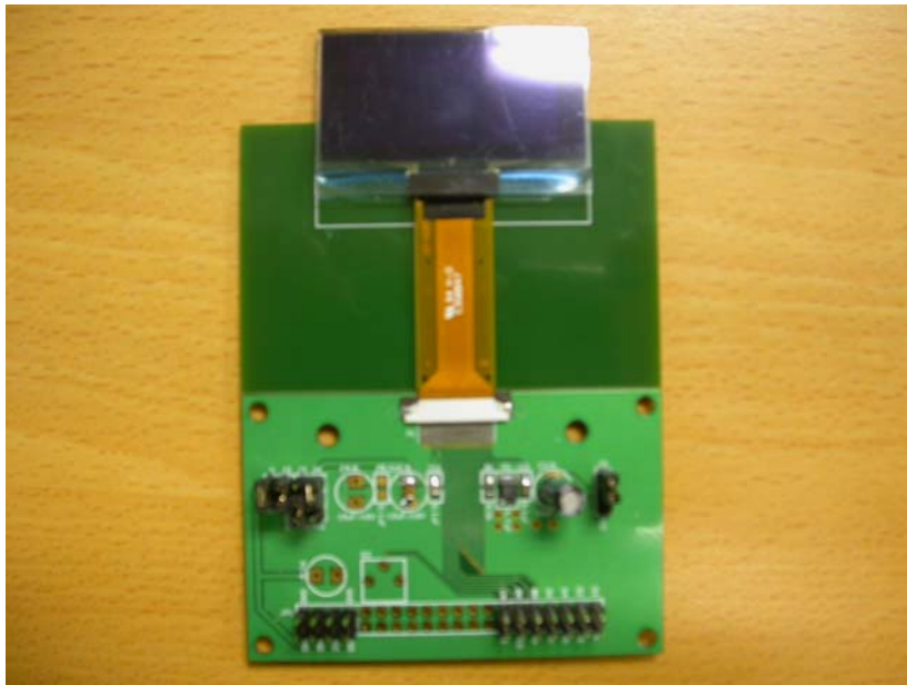
Figure 2 The combination of the module and EVK
