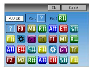
Pressing the 'Toggle' button on a toggle object allows selecting the related icons. Channels, sticks, and 2-position sticks can have 2 icons. 3 position sticks (if any) can have 3 icons. Each of the 2 (or 3) icon states can be set to empty, defining that no icon is shown for this state. The Deviation firmware comes with several predefined icons to choose from.
