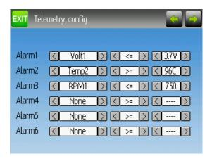
The telemetry configuration page allows specifying alarms when specific telemetry events occur.
