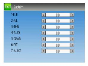
The sub-trim adjust page allows setting the zero-point of the servos for each channel. This is equivalent to the 'Sub-trim' setting on the Channel Configuration sub-page of the Mixer menu when using the Advanced GUI (see *Channel configuration*). Acceptable values range from -50 to +50 in 0.1 increments.
