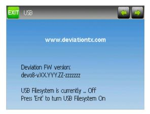
The USB page can be accessed by selecting 'USB' from the main menu. USB mode can then be toggled on/off to enable access to the transmitter's file-system from a USB equipped computer. In this mode the file system of Deviation is accessible as a mass storage device. This will allow you to move files back and forth between the Deviation file-system and a PC. All configuration files are accessible in this mode.
