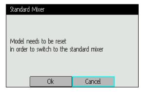
**Mixer GUI**: Defines which graphical user interface (GUI) to use for this model. The 'Advanced' GUI is the default for Deviation. The 'Standard' GUI is only available for Helicopter models and more closely resembles the stock GUI.
