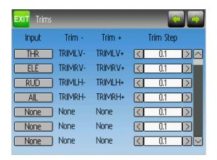
The trim page allows assigning the trim buttons and trim step, as well as configuring buttons to work as virtual inputs (see *Using a Trim as a Virtual Switch*). It is accessed from the main menu via 'Model menu' followed by 'Trims'.
