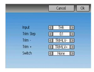
The trim-step defines how sensitive the trims are to input. The maximum number of trim steps is +/-100. So a step size of 0.1 will allow a full +/- 10% of trim adjustment on the servo.
