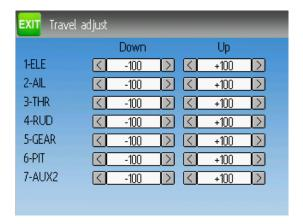
The servo-travel adjust page configures the maximum positive/negative travel of each servo. This is equivalent to the 'Scale+' and 'Scale-' settings on the Channel Configuration sub-page of the Mixer menu when using the Advanced GUI (see *Channel configuration*). Acceptable values for Down are from -175 to -1 and Up values range from +1 to +175. The default values are -100 and +100 respectively.
