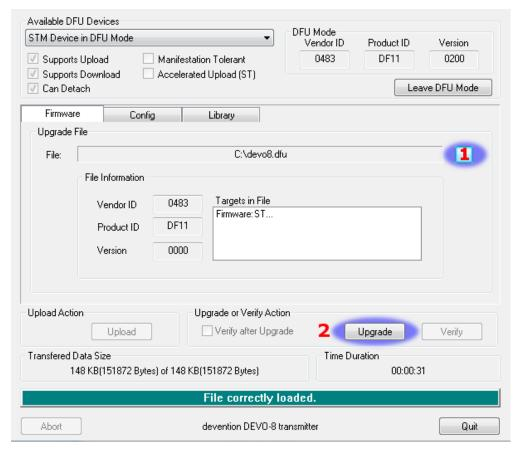
Unzip the firmware file that you downloaded earlier. Plug the transmitter into the PC via USB, and turn on the transmitter while holding 'EXT' to enter programming mode. On the Devo12, this is done by holding the trainer switch instead.
