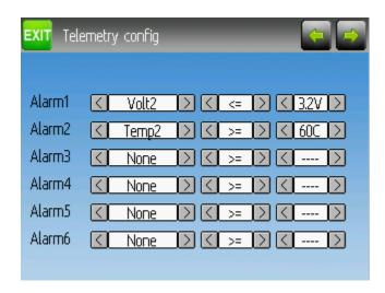
**Telemetry**: Specify the telemetry input to use for alarm control. This can be a temperature probe, voltage probe, or RPM probe.
