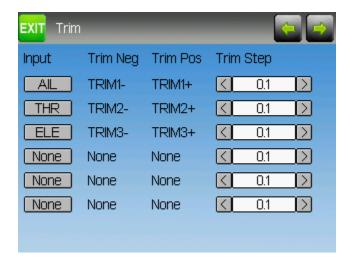
If the 'Input' field is set to an input stick, then the trim is applied as part of the mixer, and will operate as a typical trim control. If the 'Input' field is set as a channel or virtual-channel output, the value is applied directly to the channel output. In this case, the selected 'Pos' and 'Neg' buttons can operate as a virtual stick to control an output channel.
