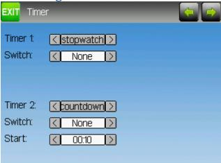
The timer page defines the 2 available timers. Timers can count either up or down, and can be enabled either manually from the main screen or by an input trigger (stick or switch)
