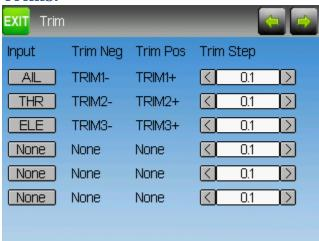
The trim page allows assigning the trim buttons an trim step. Under normal circumstances it should not be necessary to modify the trim configuration, however in some cases it may be desireable to repurpose unused trims. The Trim-step defines how sensitive the trims are to input. The maximum number of trim steps is +/-100. So a step size of 0.1 will allow a full +/- 10% of trim adjustment on the servo.
