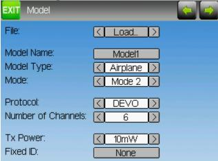
The model page allows loading and copying models, as well as loading predefined model templates. It also provides configuration options for the current model, including the Model name; Helicopter/Airplane specific configurations; Transmit Protocol; Number of channels to send to the receiver; Transmit Power; and whether a FixedID is enabled.
