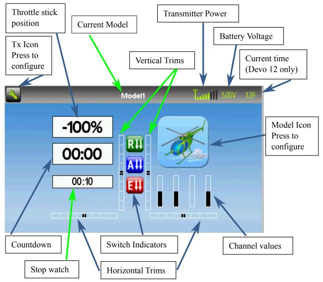
**Current Model**: The name of the current model. Clicking the label will open up the Model Load page. The model is configured from section `Model setup (Std & Adv GUI)`\_.
