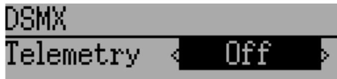
The DSMX protocol also supports enabling/disabling the telemetry capability. This option is accessed by pressing the Protocol spin-box when DSMX is shown.
