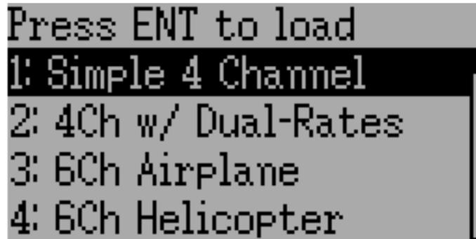
The Deviation firmware supports user-customizable predefined templates. By Selecting ‘Template...’ within the File spin-box from the Model page.
