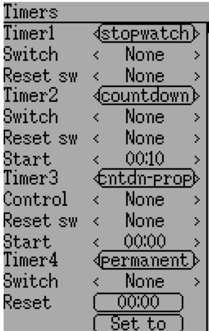
The timer page defines up to 4 available timers. Timers can count either up or down, and can be enabled either manually from the main screen or by an input trigger (stick or switch).
