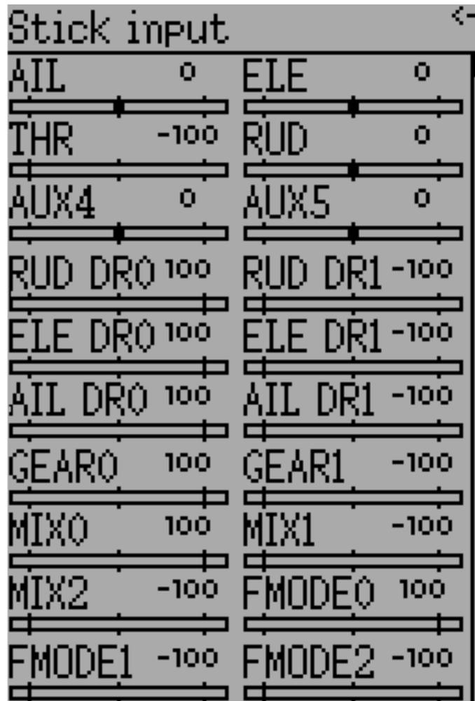
The input monitor screen shows the values associated with the current position of the control points. The values shown are a percentage of the total range of the controls based on a -100 % to +100 % scale.
