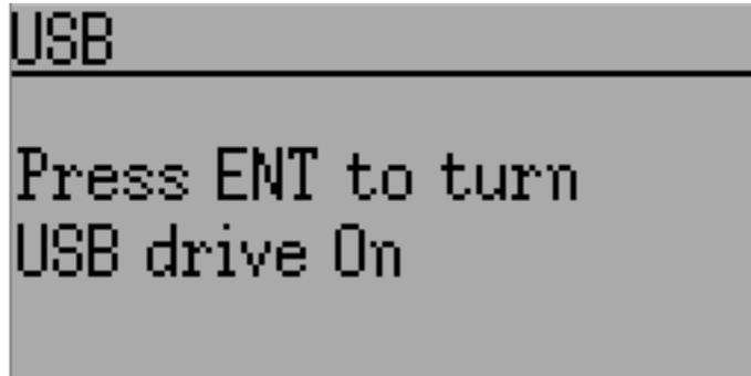
The USB page can be accessed by selecting 'USB' from the main menu. USB mode can then be toggled on/off to enable access to the transmitter's file-system from a USB equipped computer. In this mode the file system of Deviation is accessible as a mass storage device. This will allow you to move files back and forth between the Deviation file-system and a PC. All configuration files are accessible in this mode.
