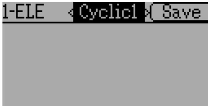
**Cyclic1, Cyclic2, Cyclic3:** The 3 outputs of the helicopter swash-plate mix. These will represent the 3 servos connected to the helicopter swash-plate (see *Swash Configuration*).
