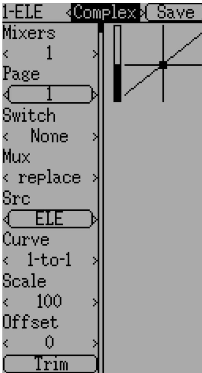
The Complex mix type unlocks the full power of the mixer system. For a given channel, any number of mixers can be applied to affect the final result. Each mixer is applied based on whether the specified switch is active, and can either replace, add to, or multiply to the previous mixers for this channel. Using this system
