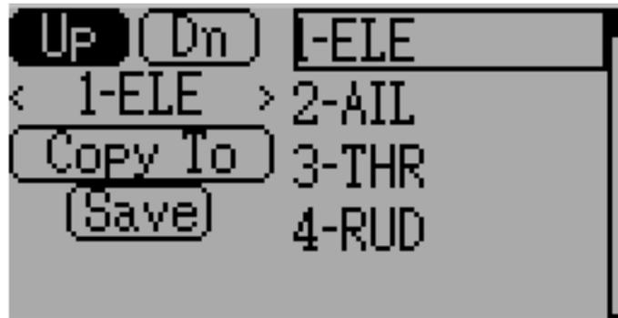
The Channel reorder page allows moving mixer definitions between channels as well as duplicating channel configurations. Note that the values displayed are the initial channel assignments. Whenever the page is loaded, the channels will be sequentially ordered representing the current state.
