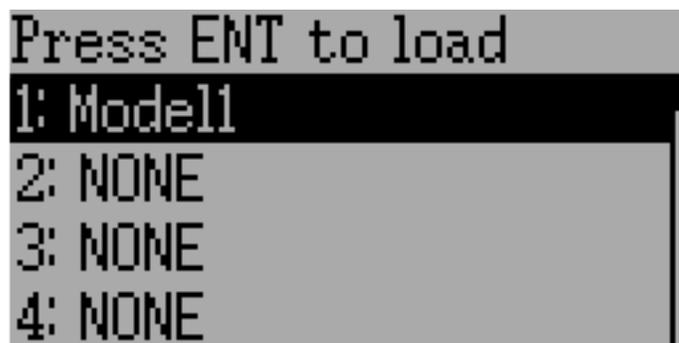
**File:** The File spin-box allows loading a new model, copying the existing model to a new location, resetting the current model to the default (all configuration is lost), and loading templates (see *Predefined Model Templates*). Note that changing models may result in a safety message being displayed (see *Safety System*).
