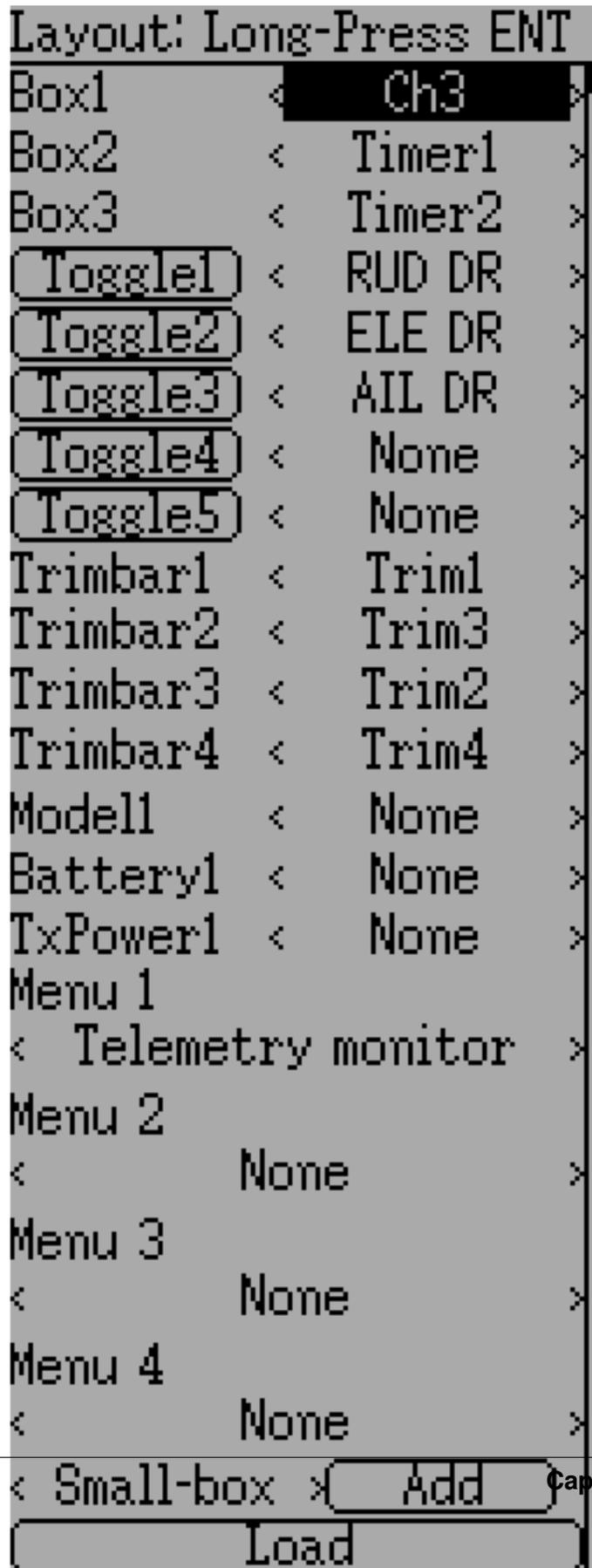
The main page config page is used to configure the main-page display. This page allows definition of which elements are shown on the main page.
