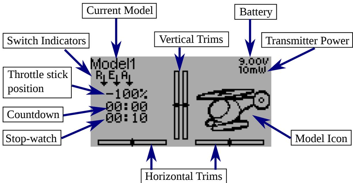
**Current Model:** The name of the current model. Clicking the label will open up the Model Load page. The model is configured from section *Model setup (Std & Adv GUI)*.
