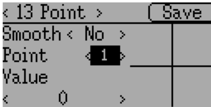
For the Multi-point curves, each point can be individually set. Points are set by choosing the point number and then choosing a value. The minimum number of points allowable is 3 the maximum number of points is 13. Enabling “Smooth” will apply a smoothing function rather than connecting points via straight lines.
