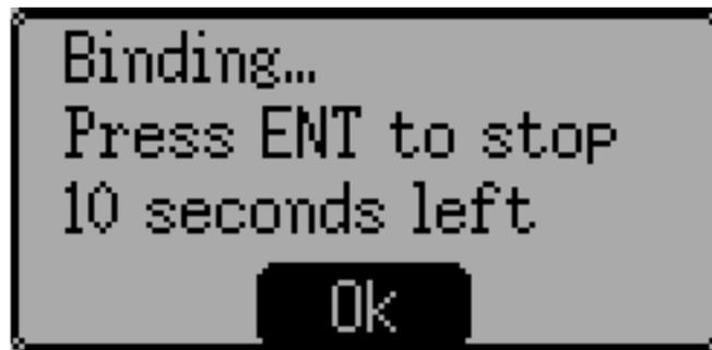
**Bind/Re-Init:** Depending on the protocol and Fixed-ID setting, the transmitter may bind with the model on start-up, or may need to be manually bound once. See *Protocols* for more on specific protocols. If the protocol does not support binding, the button will show ‘Re-Init’, which can be used to switch protocols without power-cycling the transmitter.
