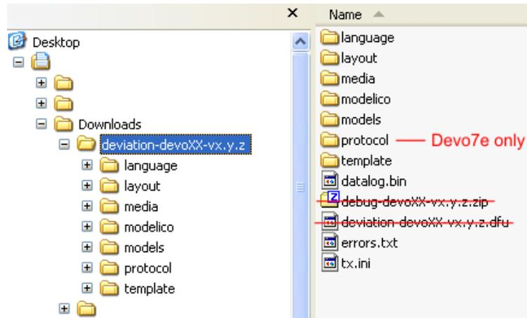
If you are upgrading from an older release, don't upgrade the “tx.ini”, and “hardware.ini” files or the “models” directory. Optionally, copy the “models” directory to the transmitter except for the currently configured model files. This last step will ensure that the defaults for newly created models have the latest options set. If the “tx.ini” file is overwritten, the stick calibration must be repeated and any settings reset.
