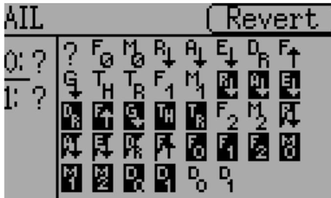
Pressing the ‘Toggle’ button on a toggle object allows selecting the related icons. Channels, sticks, and 2-position sticks can have 2 icons. 3 position sticks (if any) can have 3 icons. Each of the 2 (or 3) icon states can be set to empty, defining that no icon is shown for this state. The Deviation firmware comes with several predefined icons to choose from.
