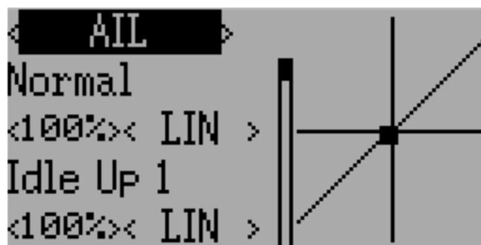
The dual-rate and expo page allows configuration of curves for the Aileron, Rudder, and Elevator channels. Up-to 3 rates can be configured for each channel, and either a scaled-linear or exponential curve can be
