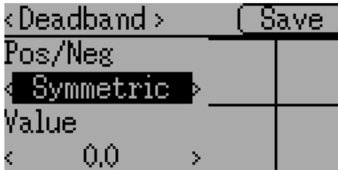
For the Deadband curve, the controls allow independently configuring the deadband width for values greater-than or less-than zero.
