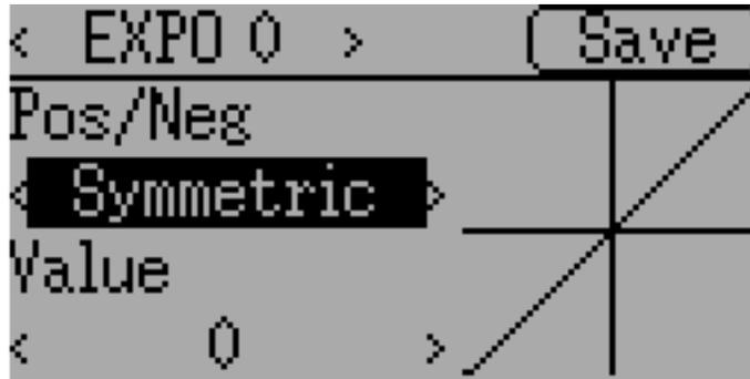
For the Expo curve, the controls allow independently configuring the shape of the curve for values greater-than or less-than zero.
