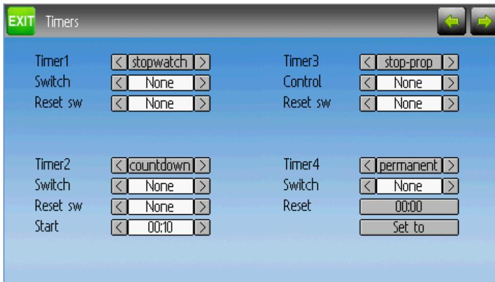
The timer page defines up to 4 available timers. Timers can count either up or down, and can be enabled either manually from the main screen or by an input trigger (stick or switch).
