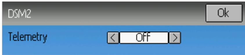
The DSM2 protocol also supports enabling/disabling the telemetry capability. This option is accessed by pressing the Protocol spin-box when DSM2 is shown.
