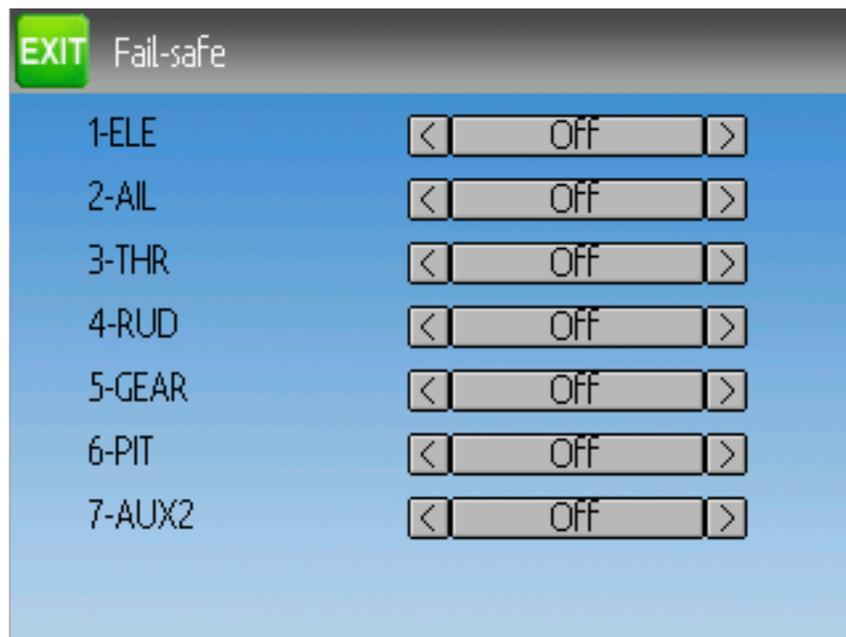
The fail-safe page is used to configure the fail-safe value for each channel (if the protocol supports this feature)
