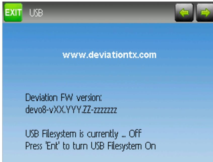
The USB page can be accessed by selecting 'USB' from the main menu. USB mode can then be toggled on/off to enable access to the transmitter's file-system from a USB equipped computer. In this mode the file system of Deviation is accessible as a mass storage device. This will allow you to move files back and forth between the Deviation file-system and a PC. All configuration files are accessible in this mode.
