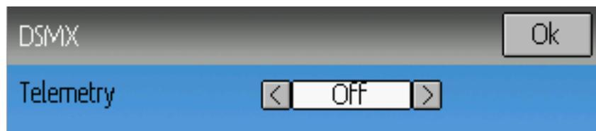
The DSMX protocol also supports enabling/disabling the telemetry capability. This option is accessed by pressing the Protocol spin-box when DSMX is shown.
