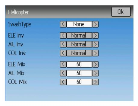
**Model Type**: Set the model-type available options are Heli, Plane and Multi. Helicopter models have an additional configuration page that can be accessed by clicking the Model type. The options for SwashType are identical to the ones in *Swash Configuration*.
