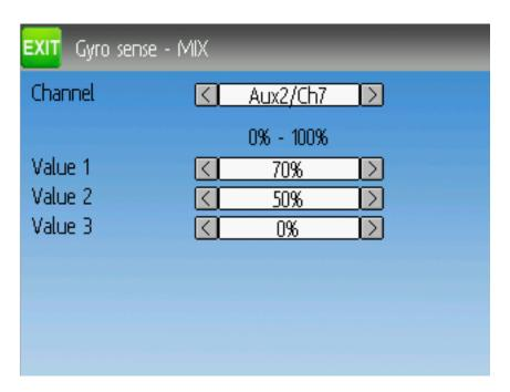
The gyro-sensitivity page enables configuring up-to 3 sensitivity values for the gyro as well as which channel to use for sending the gyro value. Acceptable values range from 0 to 100 %.
