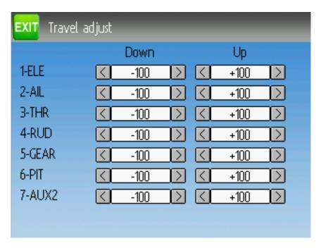
The servo-travel adjust page configures the maximum positive/negative travel of each servo. This is equivalent to the 'Scale+' and 'Scale-' settings on the Channel Configuration sub-page of the Mixer menu when using the Advanced GUI (see *Channel configuration*). Acceptable values for Down are from -175 to -1 and Up values range from +1 to +175. The default values are -100 and +100 respectively.
