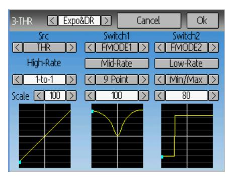
Selecting a value for Switch1 or Switch2 will activate the corresponding section. Each section can either have a "linked" curve (curve is the same as the "High-Rate" curve) in which case only the scalar can be modified, or alternatively can have an independent curve definition. Pressing the "Mid-Rate" or "Low-Rate" button for a given switch will toggle between linked and independent curves.
