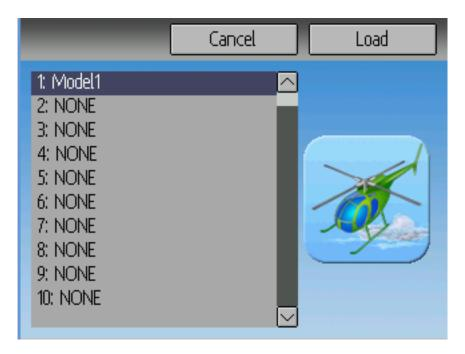
**File**: The File spin-box allows loading a new model, copying the existing model to a new location, resetting the current model to the default (all configuration is lost), and loading templates (see *Predefined Model Templates*). Note that changing models may result in a safety message being displayed (see *Safety System*).
