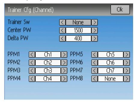
**Channel**: In channel mode, each input channel is mapped to an output channel on the instructor's transmitter. In this mode, the student's transmitter should do all necessary mixing to control the model. Care must be taken to ensure that the instructor and student transmitters are configured identically, otherwise, the model may not react well when switching between instructor and student control.
