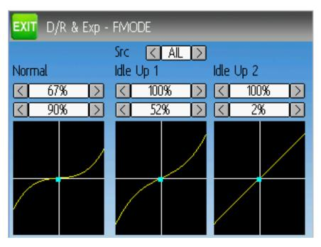
The dual-rate and expo page allows configuration of curves for the Aileron, Rudder, and Elevator channels. Up-to 3 rates can be configured for each channel, and either a scaled-linear or exponential curve can be
