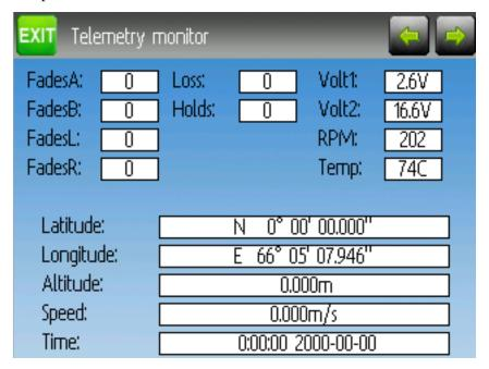
The following fields are available in DSM2 Telemetry. Note that a dedicated telemetry module and additional sensors are needed to capture this data
