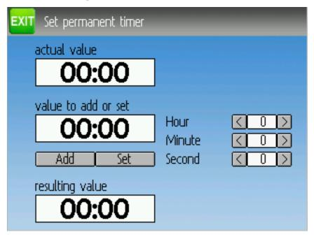
The 'permanent' timers are similar to an odometer and have their values saved in the model.ini file. They will maintain their previous value when powering up the transmitter. You can set the timer by using the "Set to" button and reset by pressing the "Reset" button.
