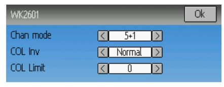
The WK2601 protocol also supports additional options. These are accessed by pressing the Protocol spin-box when Wk2601 is shown:
