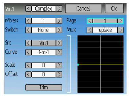
Now go to the "Mixer" page, and enter the configuration for the specified Virtual Channel (Virt1 in our example)
