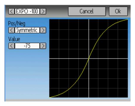
For the Expo curve, the controls allow independently configuring the shape of the curve for values greaterthan or less-than zero.
