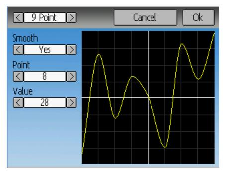
For the Multi-point curves, each point can be individually set. Points are set by choosing the point number and then choosing a value. The minimum number of points allowable is 3 the maximum number of points is 13. Enabling "Smooth" will apply a smoothing function rather than connecting points via straight lines.
