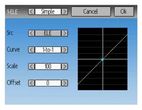
The Simple mix type is the simplest manner of defining a channel. It allows defining a primary-input (stick, switch, or other channel), and applying a curve or function to that input. The result can also be scaled or have an alternate zero-offset. You cannot use a toggle or switch to activate or deactivate this setup.
