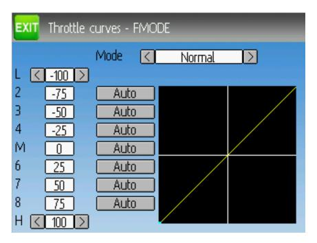
The throttle curve page allows defining a piece-wise linear curve for the throttle channel. Different curves can be selected for each flight-mode. Each point value can be enabled to be interpolated from the points surrounding it.
