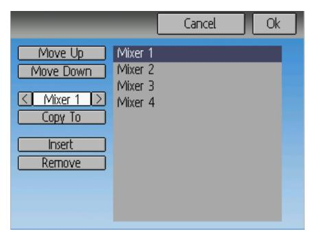
Select the respective mixer and use the up/down buttons to move the order of the selected mixer. Note that the mixer name represents its position when the reorder dialog was opened. If the dialog is closed and reopened, all mixers will be shown as numbered sequentially.
