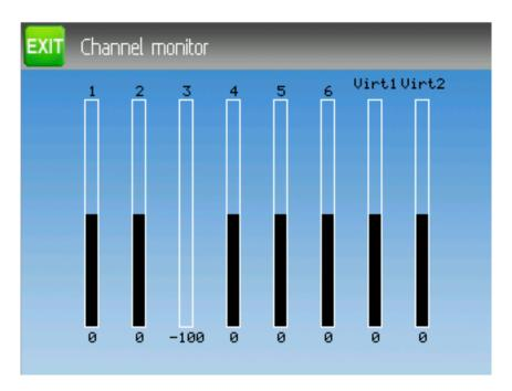
The channel monitor screen allows the user to see the values of each channel as output by the transmitter. Channels without mixers will not be displayed. Channel output displayed is the value based on minimum / maximum values as well as scaling.
