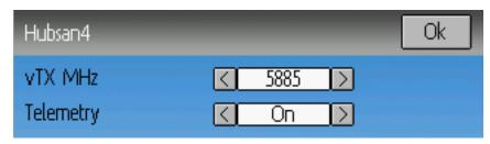
The Hubsan4 protocol supports up to 13 channels, regular format only supports auto-binding. The fixed ID can be used, but does not prevent auto-binding during power-on. The 1 st 4 channels represent Aileron, Elevator, Throttle, and Rudder. Additional channels control the quadracopter special functions:
