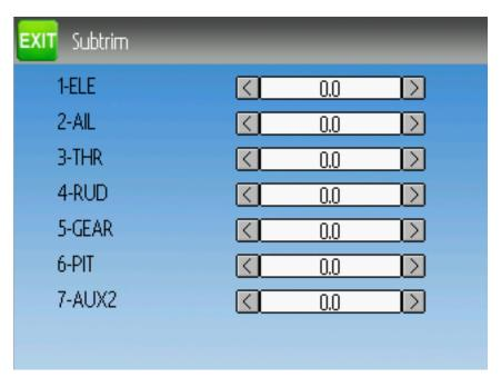
The sub-trim adjust page allows setting the zero-point of the servos for each channel. This is equivalent to the 'Subtrim' setting on the Channel Configuration sub-page of the Mixer menu when using the Advanced GUI (see *Channel configuration*). Acceptable values range from -50 to +50 in 0.1 increments.
