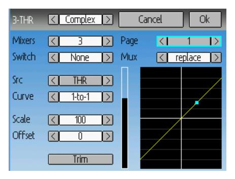
The Complex mix type unlocks the full power of the mixer system. For a given channel, any number of mixers can be applied to affect the final result. Each mixer is applied based on whether the specified switch is active, and can either replace, add to, or multiply to the previous mixers for this channel. Using this system it should be possible to define an output channel as a combination of any number of inputs.
