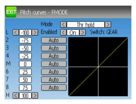
The pitch curve allows defining a piece-wise linear curve for the collective/pitch channel. Different curves can be selected for each flight-mode as well as for throttle-hold. Each point value can be enabled to be interpolated from the points surrounding it.
