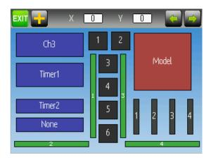
The main page config page is used to configure the main-page display. This page allows definition of which elements are shown on the main page.
