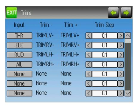
The trim page allows assigning the trim buttons and trim step, as well as configuring buttons to work as virtual inputs (see *Using a Trim as a Virtual Switch*). It is accessed from the main menu via "Model menu" followed by "Trims".
