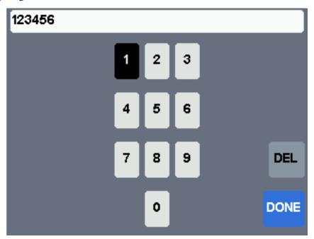
**Fixed ID**: The Fixed ID sets a unique code to ensure that the transmitter will only bind to a specific model. This is useful to ensure that the transmitter is not accidentally bound to the wrong model.
