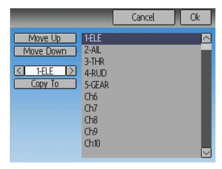
The Channel reorder page allows moving mixer definitions between channels as well as duplicating channel configurations. Note that the values displayed are the initial channel assignments. Whenever the page is loaded, the channels will be sequentially ordered representing the current state.
