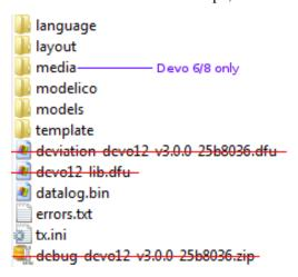
If you are upgrading from an older release, don't upgrade the "tx.ini", and "hardware.ini" files or the "models" directory. Optionally, copy the "models" directory to the transmitter except for the currently configured model files. This last step will ensure that the defaults for newly created models have the latest options set. If the "tx.ini" file is overwritten, the stick calibration must be repeated and any settings reset.
