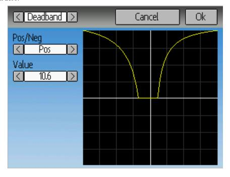
For the Deadband curve, the controls allow independently configuring the deadband width for values greaterthan or less-than zero.
