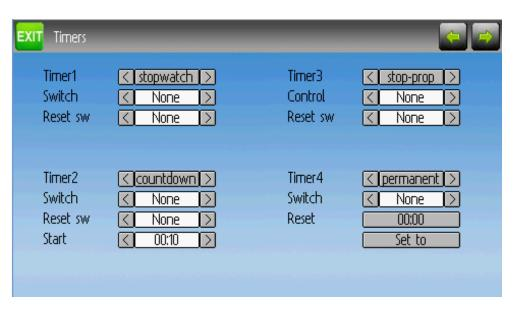
The timer page defines up to 4 available timers. Timers can count either up or down, and can be enabled either manually from the main screen or by an input trigger (stick or switch).
