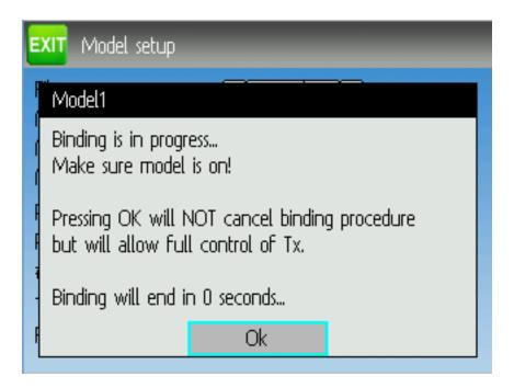
**Bind/Re-Init**: Depending on the protocol and Fixed-ID setting, the transmitter may bind with the model on start-up, or may need to be manually bound once. See *Protocols* for more on specific protocols. If the protocol does not support binding, the button will show 'Re-Init', which can be used to switch protocols without power-cycling the transmitter.
