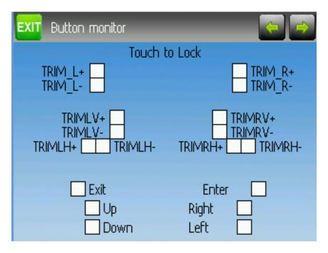
The button monitor page is used to ensure physical buttons on the transmitter are working as expected. Pressing any physical button will select the corresponding square on the screen. To test 'EXT', 'L-' or 'R+' touch the screen to disable menu traversal. Touch the screen again to unlock.
