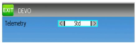
The DEVO protocol also supports enabling/disabling the telemetry capability. This option is accessed by pressing the Protocol spin-box when DEVO is shown. The options are Std (standard format), X350 (Walkera QR-X350 format), and Off.
