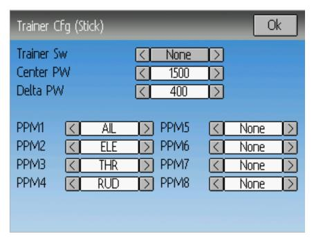
**Stick**: In stick mode, each input channel is mapped to a stick on the master transmitter. In this mode, the student moving the stick will behave exactly as if the instructor had moved the stick. Generally when using this mode, the student's transmitter will directly pass the stick position (no mixing) and the instructor's transmitter will do all necessary mixing.
