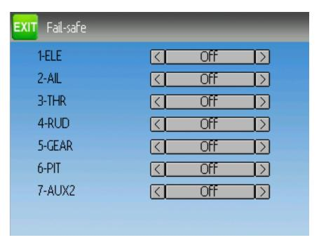
The fail-safe page is used to configure the fail-safe value for each channel (if the protocol supports this feature)
