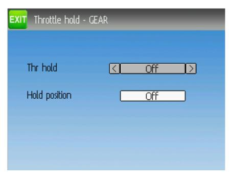
The throttle-hold page is used to enable/disable the throttle-hold capability. Specifying 'Hold position' defines the throttle value when the Throttle-hold switch is set. Hold position can be set from -200 to 200.
