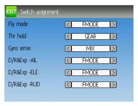
The switch assignment page enables configuring which switches to use for each capability in the standard-GUI. The same switch may be assigned to multiple capabilities.
