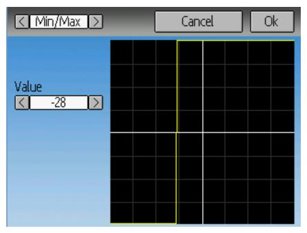
For the Min/Max, Zero/Max, >0, <0, and ABSVAL, the controls allow setting the transition point along the x-axis. A value of '0' will be symmetric around the y-axis, positive or negative values will move the center point accordingly
