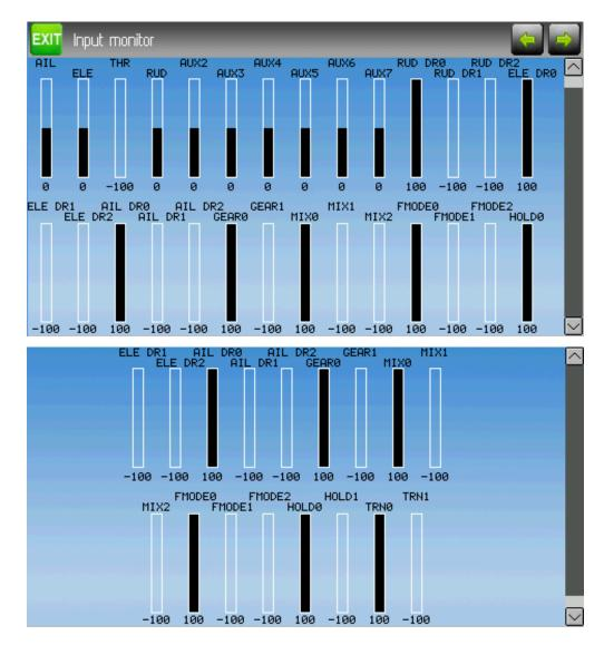
The input monitor screen shows the values associated with the current position of the control points. The values shown are a percentage of the total range of the controls based on a -100% to +100% scale.
