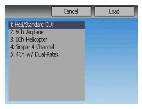
The Deviation firmware supports user-customizable predefined templates. By Selecting 'Template...' within the File spin-box from the Model page.
