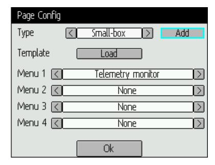
Select the "+" icon to open the add-item dialog. Then select the object type from the spin-box on the left, then press 'Add' to create the object. This will add the specified object type to the center of the screen. You can now place and configure the new object.
