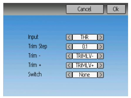
The trim-step defines how sensitive the trims are to input. The maximum number of trim steps is  $\pm$ 100. So a step size of 0.1 will allow a full  $\pm$ 10% of trim adjustment on the servo.
