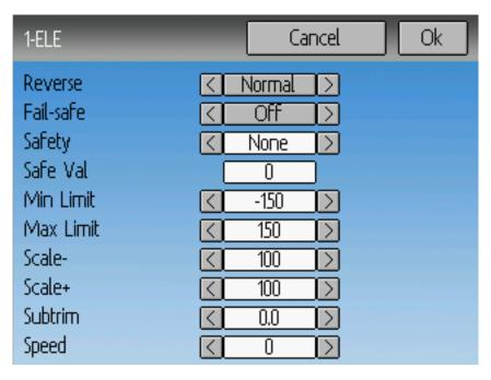
The Channel configuration provides the ability to configure the final channel outputs. Capabilities such as channel reverse and fail-safe values are applied here. Also available are controls for end-points, scaling,
