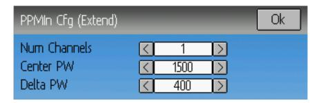
Deviation has the ability to use PPM input signals from an external source (such as an FPV setup). To configure this mode, set the PPM In mode to 'Extend' in section *Model setup (Std & Adv GUI)*.
