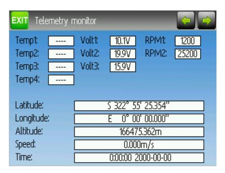
Certain protocols have the ability to transmit telemetry data back to the transmitter during use. Telemetry data may include, but is not restricted to, temperature readings, various voltage readings, motor or engine rpm, as well as GPS related information.
