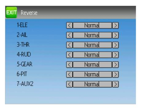
The servo reverse page allows quickly setting each channel to work in either normal or reversed mode. These settings are equivalent to the 'Reverse' setting on the Channel Configuration sub-page of the Mixer menu when using the Advanced GUI (see section *Channel configuration*)
